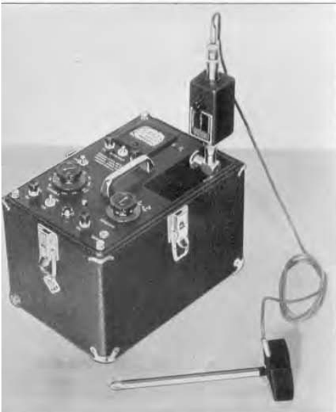
FIGURE 20. The control box and vibration pickup connect to the sound-level meter in place of the microphone.
